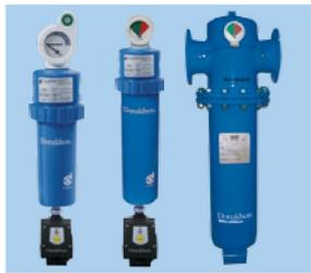
**Filter Housings** • Flow rate from 1440 m<sup>3</sup>/hr to 2880 m<sup>3</sup>/hr (AG) and from 1080 m<sup>3</sup>/hr to 38400 m<sup>3</sup>/hr (SG) • Low pressure drop • Include differential pressure gauge and condensate drain • SG available with ATEX specification • Maximum working pressure 16 barg
