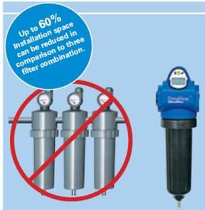
**(Three) Stage Filter** This unique filter element combines 3 high efficiency purification stages in one single element. • Sub-Micro coalescence filter • Activated carbon adsorbent • High efficiency particle filter (class 1 acc. to ISO8573-1:2010) • Nominal flow rates up to 110 m<sup>3</sup>/hr @ 7 barg • Economiser offers control of filter lifetime and differential pressure • Compact space saving solution for point of use application • Service advantages vs. multiple housing combination
